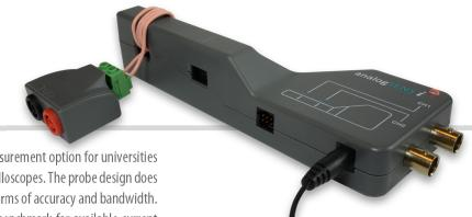
analogSENS probes are designed to create a very low cost current measurement option for universities with low budgets. They can be interfaced to all types and brands of oscilloscopes. The probe design does not compromise on quality and beats much higher cost alternates in terms of accuracy and bandwidth. The specifications of the probe truly defines a new value for money benchmark for available current probes in the market.
